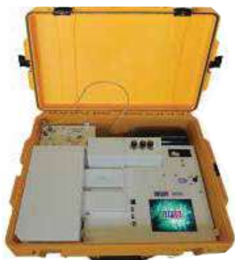
Companion 2 portable GC (with Headspace Concentrator)
